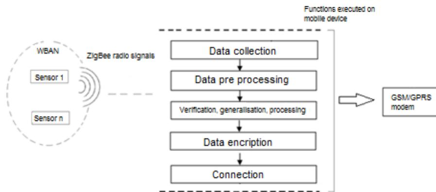
Figure 3. Display of processes running on sensor data
