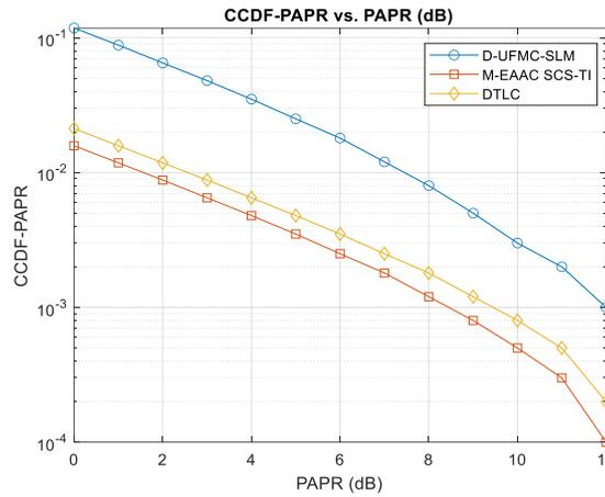
Figure 6. CCDF-PAPR vs. PAPR (dB) between: 1) D-UFMC-SLM, 2) M-EAAC SCS-TI and 3) DTLC under No. of transmitting antennas (N=2), Subblocks (M)= 8, 16 and 32
