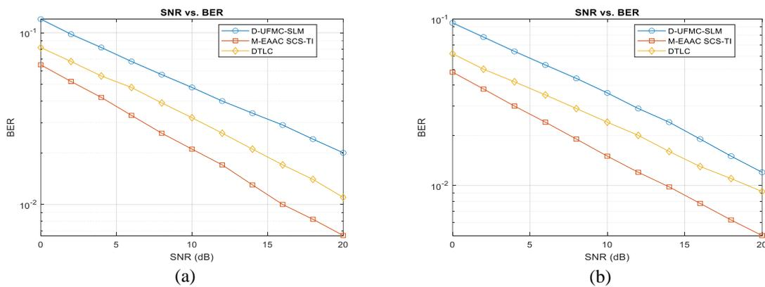
Figure 9. BER vs. SNR (a) under phase vector 7 (b) under phase vector 9 between: 1) D-UFMC-SLM, 2) M-EAAC SCS-TI and 3) DTLC under various phase vector with M-ary QAM encoding with FFT  $N_{sc} = 1024$
