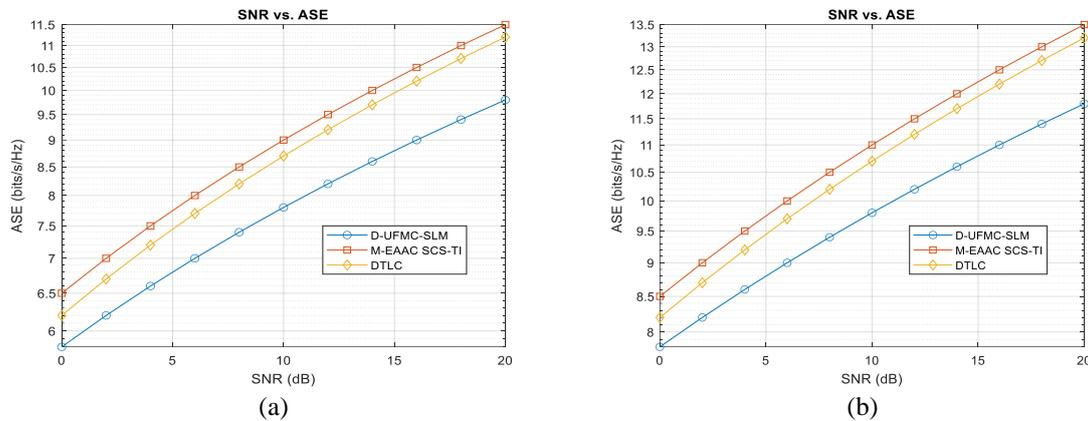
Figure 10. Average Spectral Efficiency between: 1) D-UFMC-SLM, 2) M-EAAC SCS-TI and 3) DTLC vs. SNR under M-ary encoding QAM (a)32 and (b) 64
