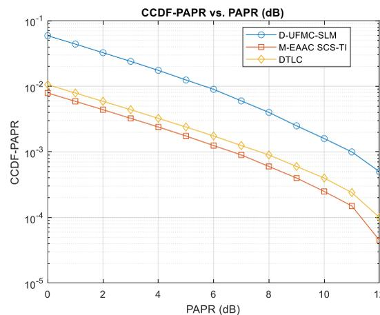
Figure 7. CCDF-PAPR vs. PAPR (dB) between: 1) D-UFMC-SLM, 2) M-EAAC SCS-TI and 3) DTLC under No. of transmitting antennas (N=4), Subblocks (M)= 8, 16 and 32
