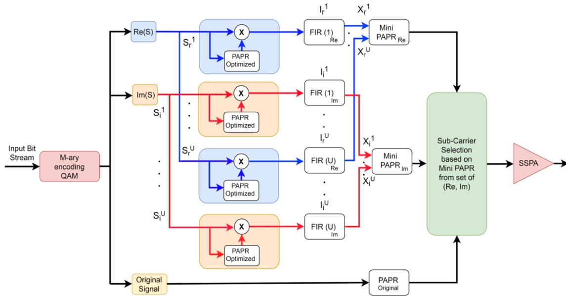
Figure 3. Block diagram of -UFMC-SLM
