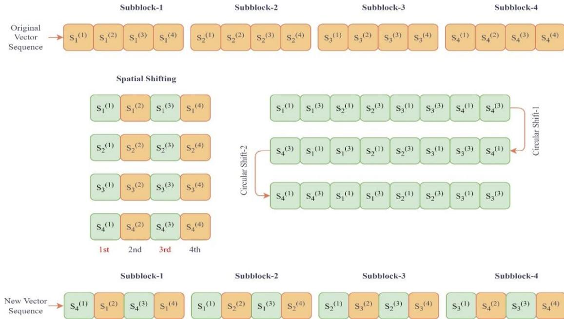
Figure 5. SCS-TI in decomposed SLM technique
