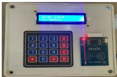
Figure 3. Door access control artifact
