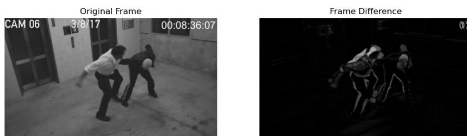
Figure 4. Frame difference information extracted by using change detection technique
