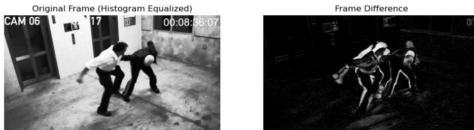
Figure 5. Frame difference information extracted after using histogram equalization
