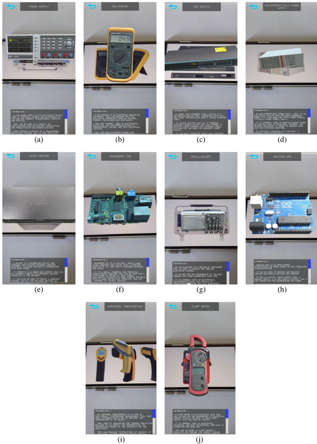
Figure 7. Image tracker output for: (a) power supply, (b) multi-meter, (c) Poe switch, (d) Ups power, (e) Cisco router, (f) Raspberry Pi, (g) Oscilloscope, (h) Arduino Uno, (i) infrared thermometer, and (j) clamp meter
