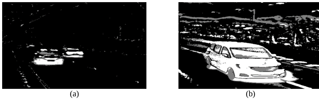
Figure 9. Foreground extraction results using background subtraction for (a) nighttime and (b) daytime
