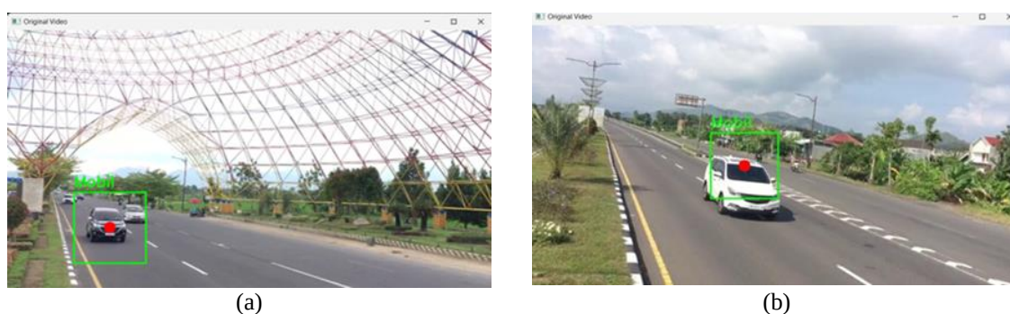
Figure 11. Vehicle detection results using Haar cascade for (a) nighttime and (b) daytime
